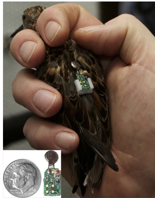
Figure 4. Accelerometer tag mounted to sandpiper and tag with US dime for scale (insert).
